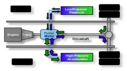
Fig 3: Hydraulic assisted RBS
